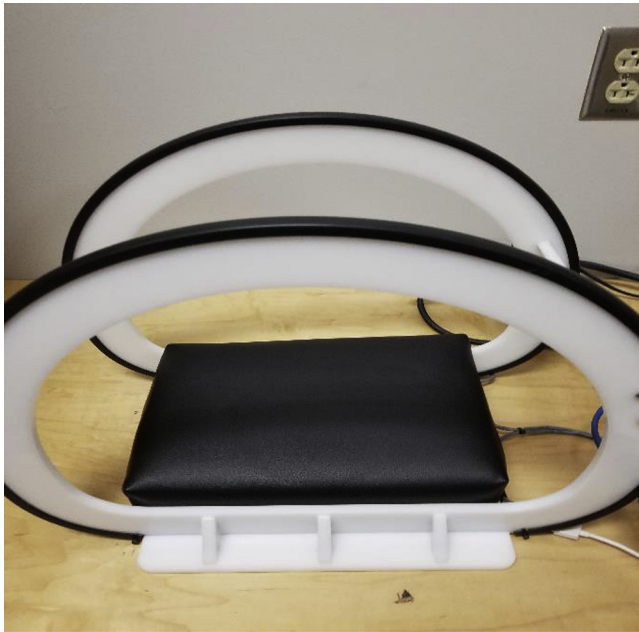
Figure 1 Study device. The device is designed for the patient's head and upper neck to lie in the center of the electromagnetic field created by the Helmholtz coil situated around the headrest. The device connects to an external stimulator, which provides the specified field strength and stimulation frequency.
